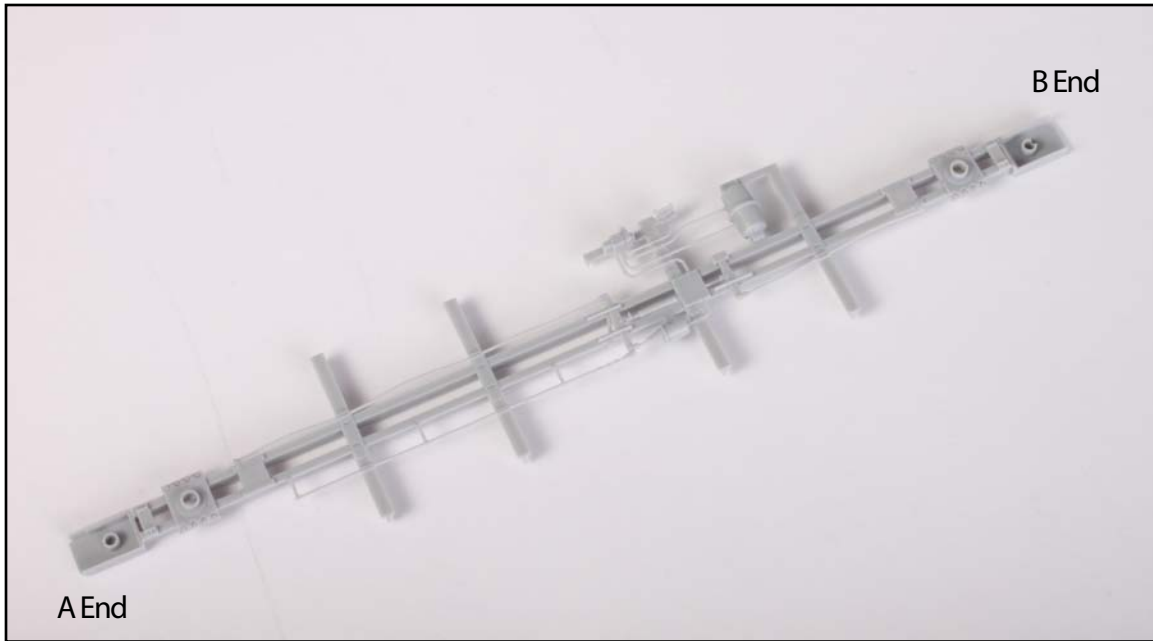
Photo A: Under Frame
